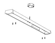
If mounting to junction box, place fixture against junction box and install two (2) screws through junction box mounting holes and into junction box mounting tabs.
