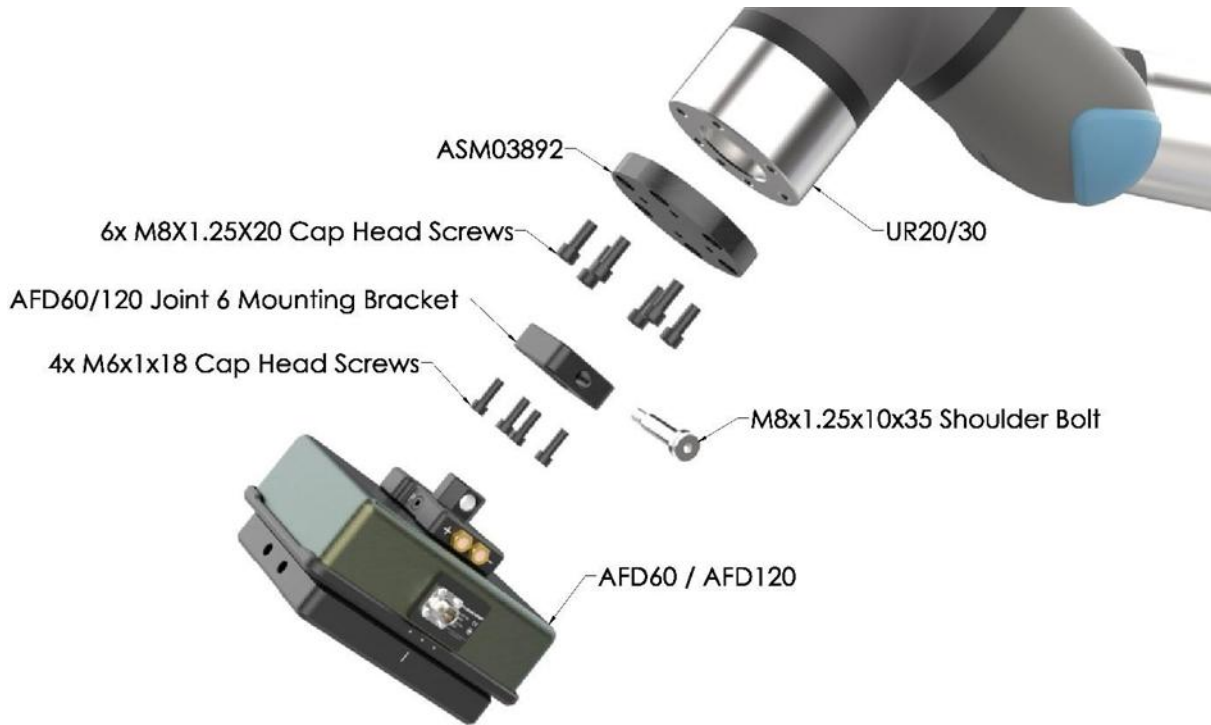
Figure 7: AFD62/120 Mouning to Joint 6 of UR20/30
