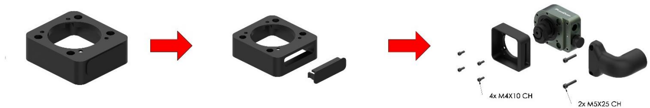
FIGURE 5: DUST COLLECTION TAB REMOVAL
