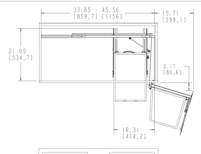
\*NOTE: THIS UNIT IS DESIGNED FOR FRAMELESS CABINETS. IF INSTALLING IN FACE FRAME CABINETS THE SIDE WALL AND FLOOR NEEDS TO BE FLUSHED OUT.
