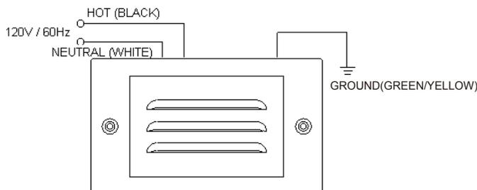
2) Insert Fixture into the Wall Single-Gang Box. Secured with mounting screws(2).
