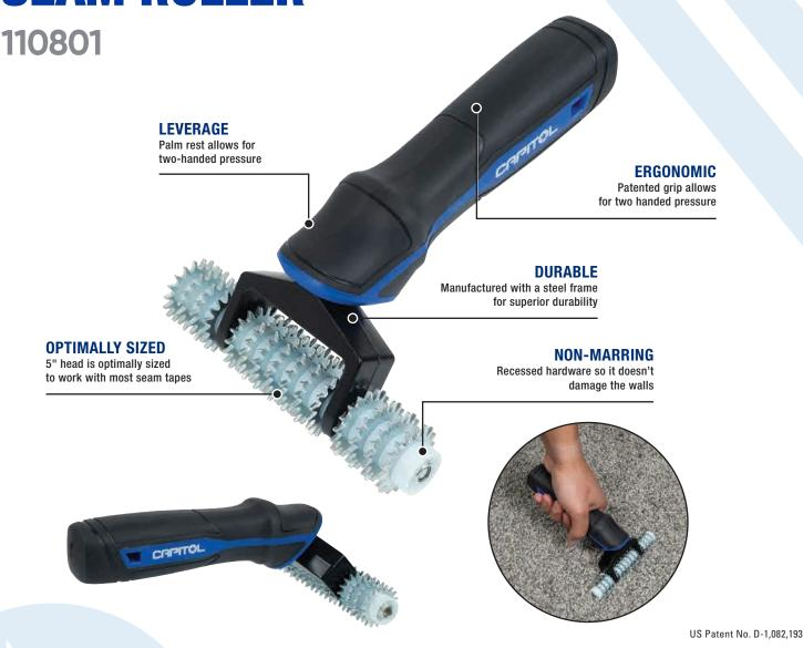
Capitol® Star Wheel Loop Pile Seam Roller is specifically designed for seaming loop pile and Berber carpets. It features star wheels to maximize the transfer of hot-melt tape into the carpet and produce stronger seams. It has a longer handle and palm rest on top of the rugged steel frame to provide optimum leverage and durability.
