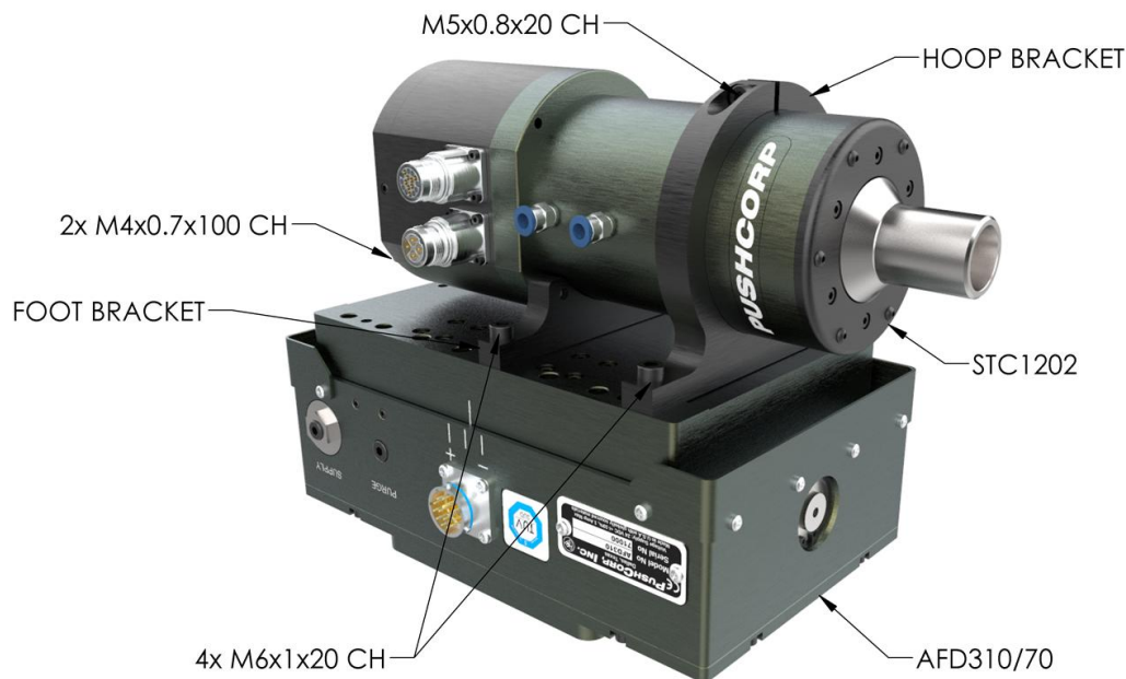
FIGURE 1: PARALLEL MOUNT - AFD310/70
