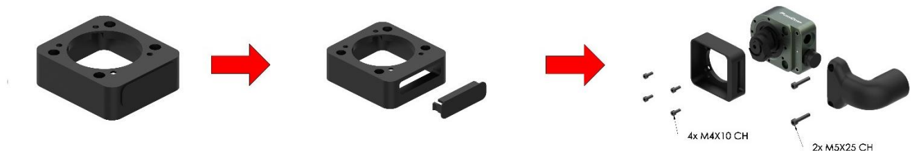
FIGURE 5: DUST COLLECTION TAB REMOVAL
