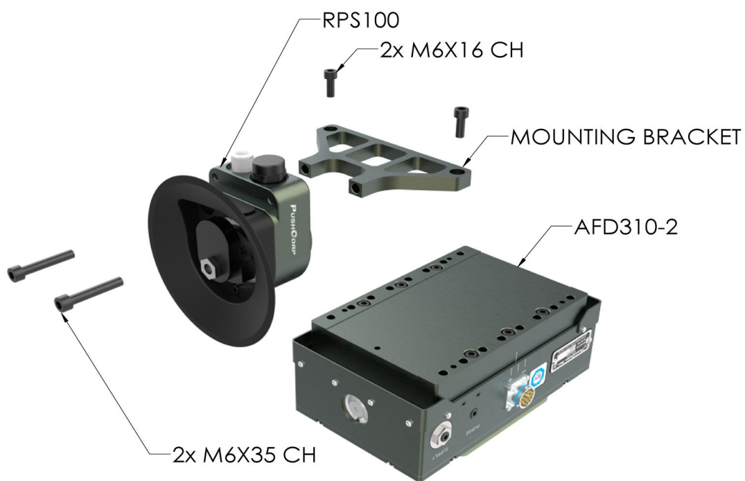
FIGURE 2: RPS100-AFD310-2 MOUNTING CONFIGURATION
