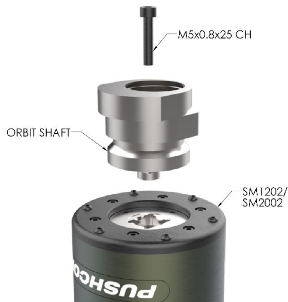
FIGURE 12: ORBIT ASM ASSMEBLY STEP 1
