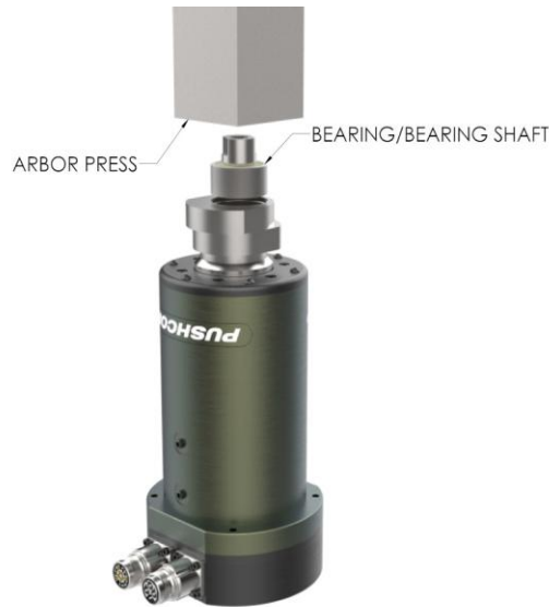
FIGURE 13: ORBIT ASM ASSEMBLY STEP 2
