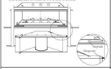
6 Hook the safety cables into the holes located on the end brackets. Connect wiring as shown. Pink and purple wiring are for 1-10V dimming systems. Cap off if not used.
