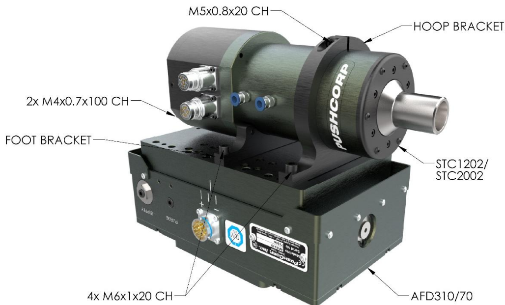
FIGURE 1: PARALLEL MOUNT - AFD310/70
