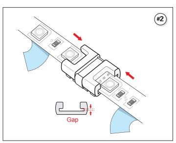
Insert FlexTape® into slots on both ends until fully seated
