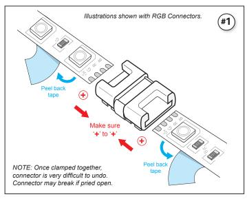
Peel back FlexTape® backing. Be sure to match polarity (+ to +)
