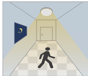
With insufficient ambient brightness, light dims to 100% when motion detected.
