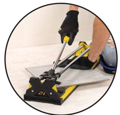
**CUTS CERAMIC, PORCELAIN AND MOSAIC FLOOR AND WALL TILE UP TO 21" LONG, 15" DIAGONALLY AND 3/8" THICK**
