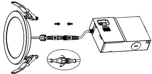
If using extension cables, insert cable between driver and fixture ensuring the connectors are properly aligned and fully screwed down.
