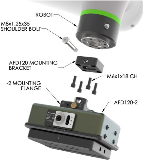
Figure 5: AFD120-1 Mounting
