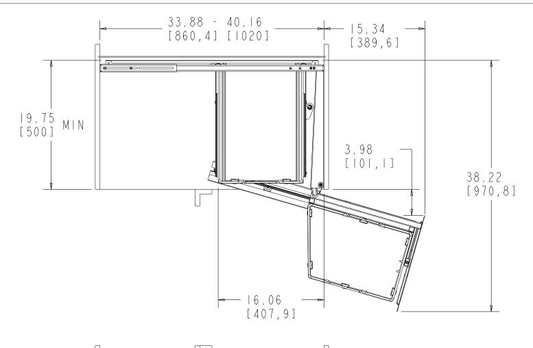
\*NOTE: THIS UNIT IS DESIGNED FOR FRAMELESS CABINETS. IF INSTALLING IN FACE FRAME CABINETS THE SIDE WALL AND FLOOR NEEDS TO BE FLUSHED OUT.
