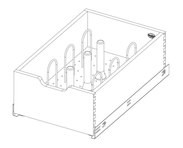
NOTE: THIS DRAWER IS MADE FOR PILASTER SYSTEM AND THE CABINET DIMENSIONS BELOW ARE FOR THE DRAWER AND PILASTERS.
