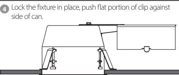
NOTE: In areas where excessive ceiling vibration can occur, we suggest you use a #1/4-14 x 1/2" pan head sheet metal screw to further lock the spring clips against the fixture housing. Drive the screw through the hole in the spring clip and into the housing slot. To remove the housing from the ceiling, pull down on the clip.
