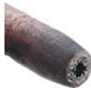
Nozzle fully clogged (not using E-WELD NOZZLE MC )
