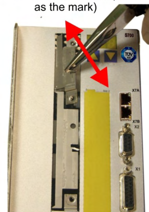
6 - Pull out the top plate
