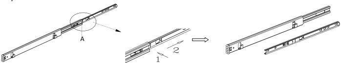
Step 2: SCREW INNER SLIDE TO THE PARTITION WALL.
