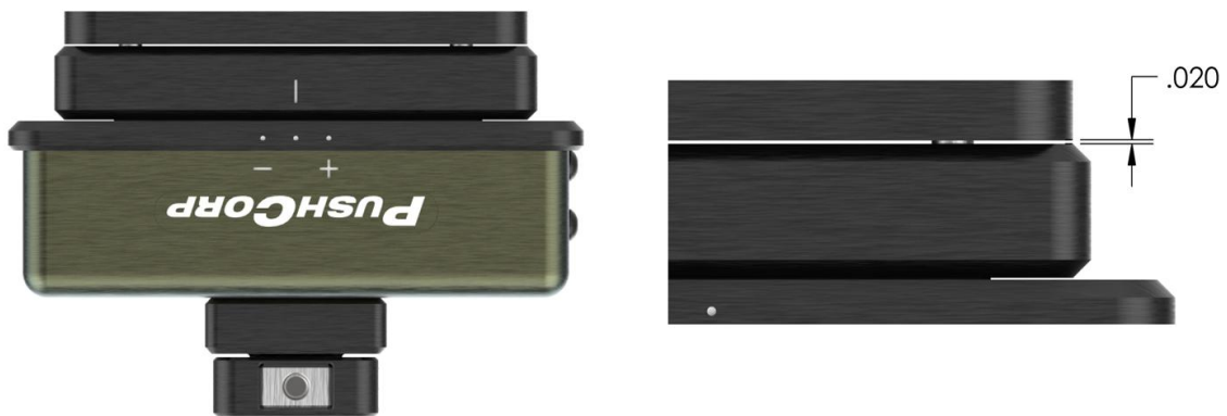
Figure 3: Carriage Mount Bracket - Shims
