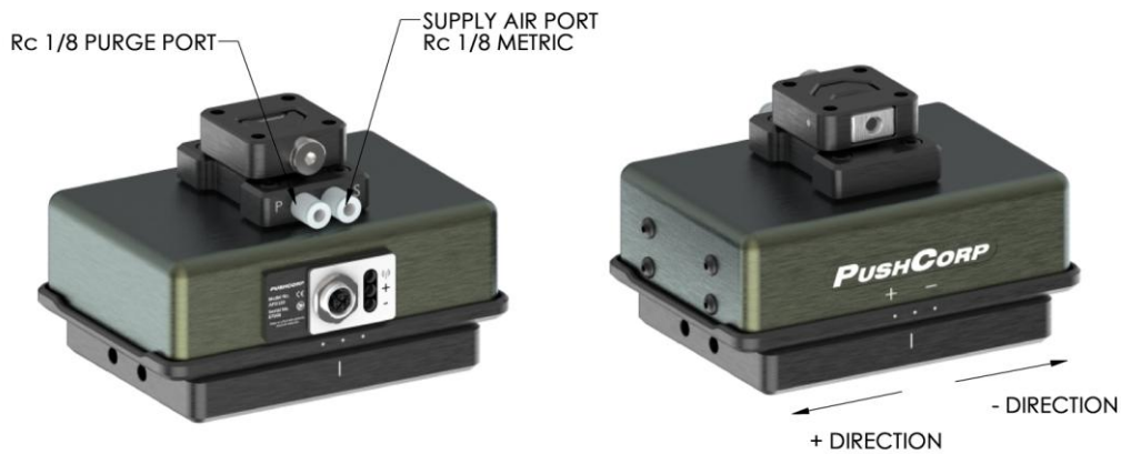
Figure 9: AFD120 Air Connections
