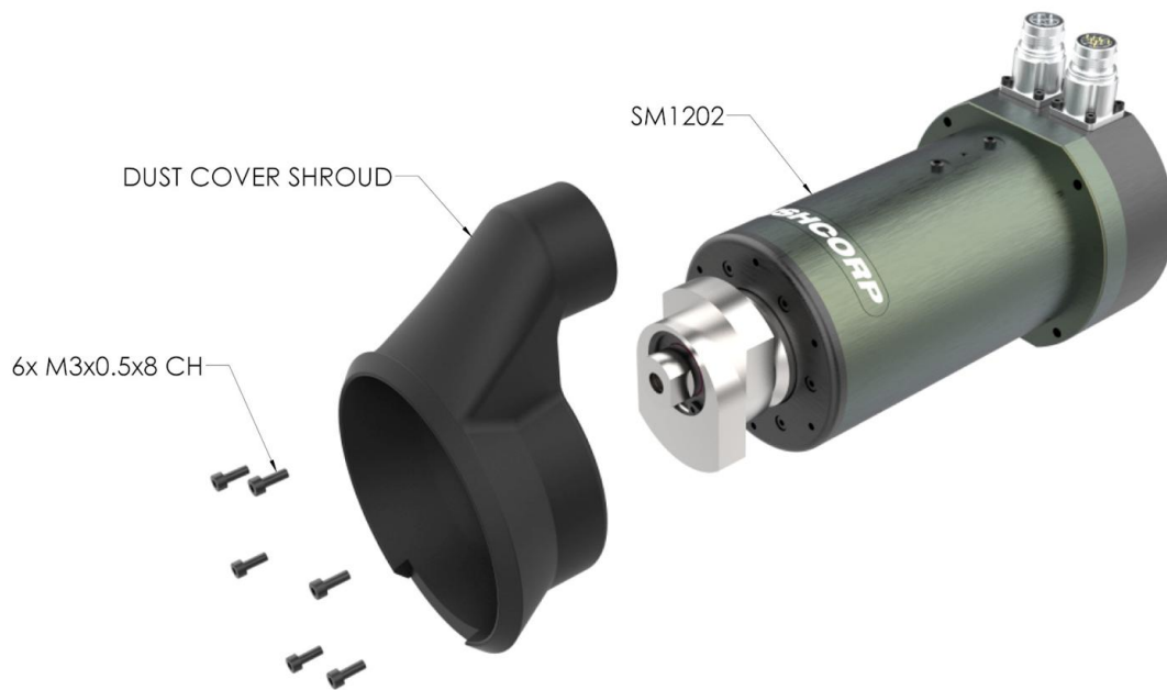
FIGURE 6: DUST SHROUD INSTALLATION STEP 2
