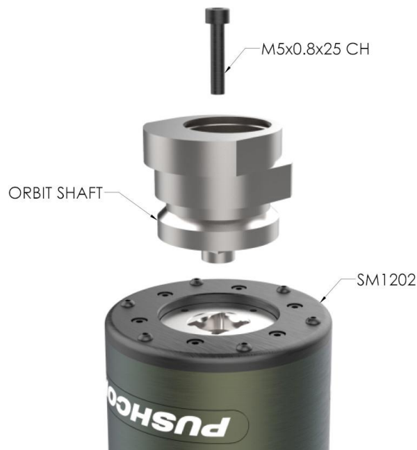
FIGURE 12: ORBIT ASM ASSEMBLY STEP 1
