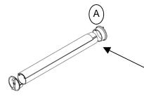
4. Take the end with the  $\frac{1}{2}$ " exposed rod and insert into full circle pole cup. See figure A.
