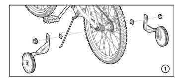
**A** WARNING: The inner axle nut which holds the rear wheel on should not be removed or loosened while installing the training wheels (see Figure 1).
