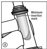
WARNING: Do not over tighten the stem bolt. Over tightening the stem bolt can damage the steering system and cause a loss of control. If necessary re-adjust the handlebar and tighten the handlebar clamp nut.
