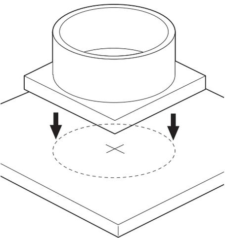
Align Drill Guide over marked surface and press firmly.
