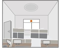
When ambient brightness is lower than preset lux level, sensor will turn on light automatically and keep dimming according to the change of the ambient brightness; when outside is getting darker, the inside will be brighter, and brighter darker.
