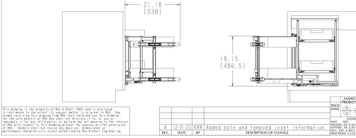
\*NOTE: THIS UNIT IS DESIGNED FOR FRAMELESS CABINETS. IF INSTALLING IN FACE FRAME CABINETS THE SIDE WALL AND FLOOR NEEDS TO BE FLUSHED OUT.
